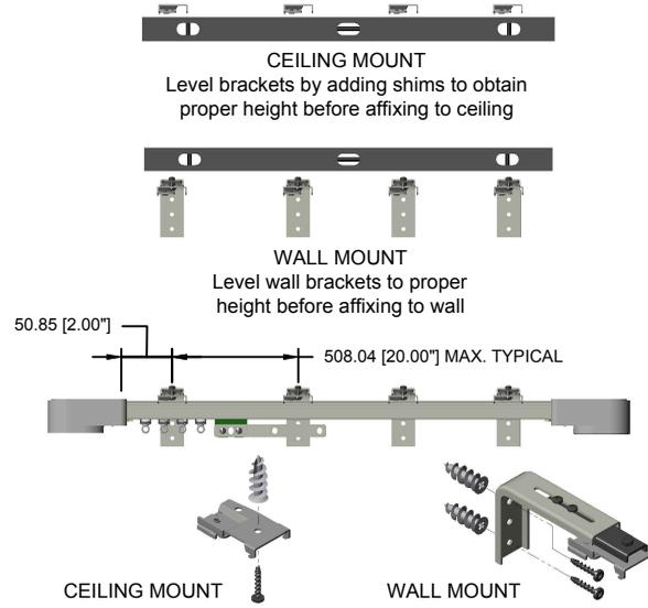
Note: Installer to provide wall anchors and screws appropriate to the surface material and weight of the product. Metal, self-drilling anchors are recommended for drywall.
