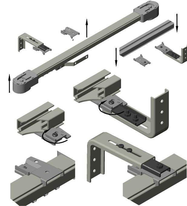
4. Attach fabric wrap clip for fabric return (If Desired).
