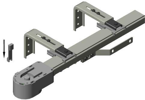
5. Slide motor drive shaft into drive gear and secure the locking clip. Locking clip must be fully engaged by sliding lever past the locking mechanism.
