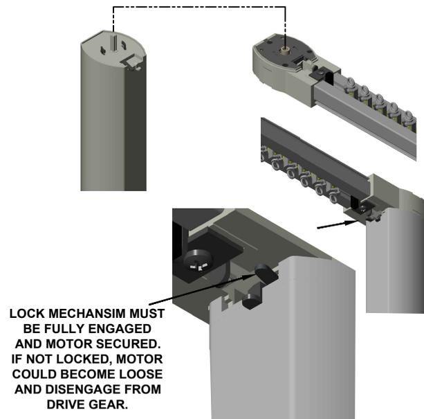
**LOCK MECHANISM MUST BE FULLY ENGAGED AND MOTOR SECURED. IF NOT LOCKED, MOTOR COULD BECOME LOOSE AND DISENGAGE FROM DRIVE GEAR.**
