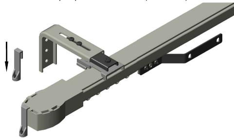
4. Installing Solar Panel and Brackets. Solar Panel **MUST** be exposed to Direct Sunlight and Inside the window, and mounted in close proximity to Solar Motor.
