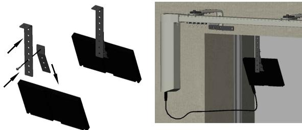
5. Slide motor drive shaft into drive gear and secure the locking clip. Locking clip must be fully engaged by sliding lever past the locking mechanism.
