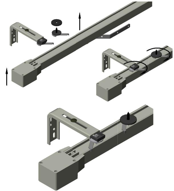
4. Attach fabric wrap clip for fabric return. Fabric clip is opposite from Motor Latch as seen below.
