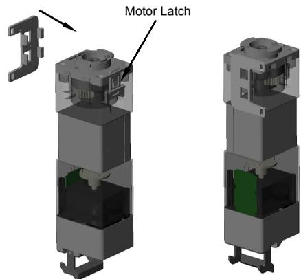
5. Align Blue Dot on Drive Gear Head with Blue Dot on Drive Motor. Slide Drive Motor into Drive Gear Head and rotate 90° clockwise. Slide Motor latch up into Drive Gear Head completely until latch locks into place. Latch must be fully engaged by sliding lever past the locking mechanism until it clicks.
